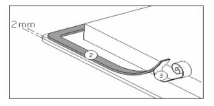
Stick the gasket (2) two millimeters from the external edge of the glass, after removing the protection tape (3).
