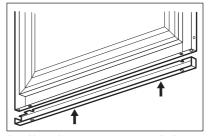
**3.** Align the compensator with the steel door panel and tighten the screws.
