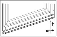
**4.** Insert the steel carter inside the compensator as indicated in the figure.
