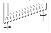
Position the steel compensator as indicated in the figure and insert the upper part under the head of the screws.
